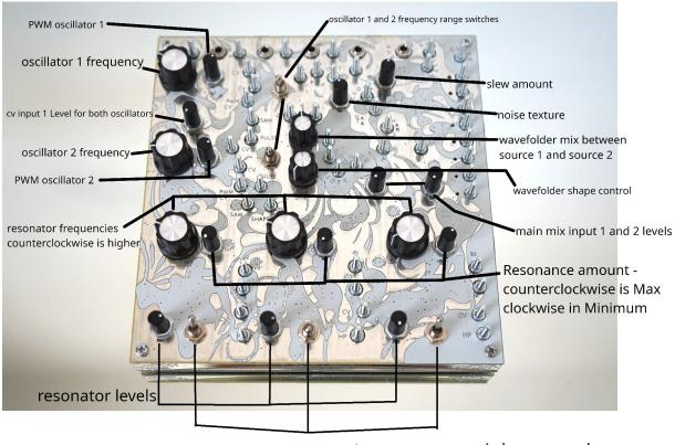
resonator response: up is low pass , down is band pass
